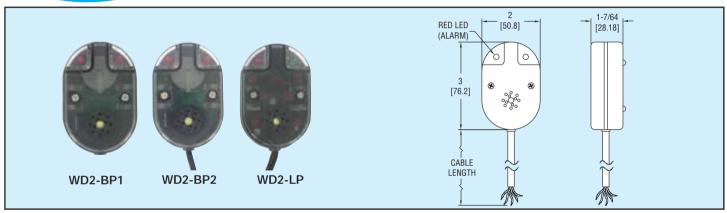
Protect your equipment from water leaks. The WD2 Water Leak Detector detects leaking water and sounds an alarm before the leak turns into a costly mess. The WD2 relies on the electrical conductivity of water to change the resistance across the two contacts located at the base of the enclosure. The Model WD2-BP1 and WD2-BP2 are standalone battery powered units and are provided with audible and visual alarms, plus low battery warning. The Model WD2-BP2 includes a solid state relay output.
