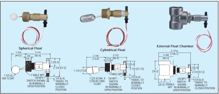
The Mini-Size Series L10 Flotect\* Level Switches combine low cost with top quality materials and construction for great value and years of reliable liquid level control. Wide media compatibility is assured with a choice of brass or stainless steel bodies and external tees; polypropylene or stainless steel floats. Two basic configurations are offered; with 1" male NPT threads for direct side mounting through a half coupling or with factory installed tee for external mounting.
