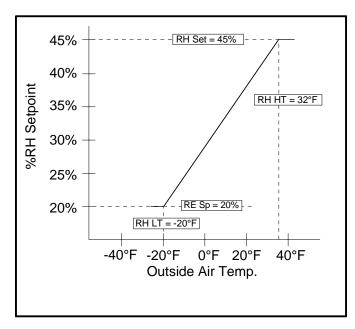
Fig.11 – Humidity setpoint reset by outside air temperature
