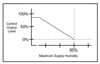
Fig. 12 - High humidity limit vs Control output level curve
