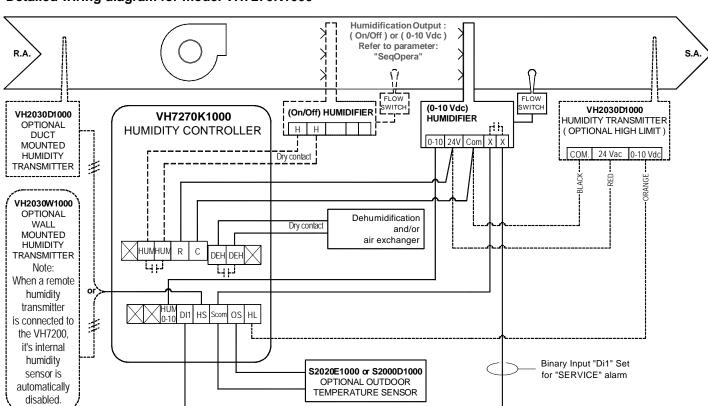
Fig.6: VH7270F1000 wiring diagram
