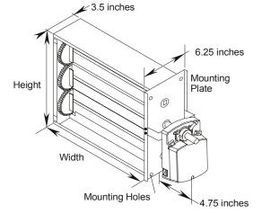
Figure 2: Damper Dimensions, inches
