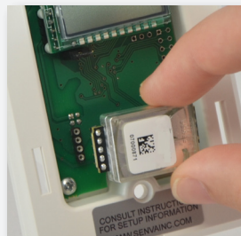
Field replaceable CO2 NDIR element
